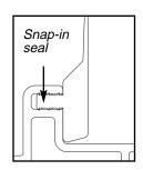
Swinging door models have bottom track with snap in seal.
